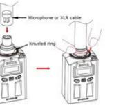
Push the microphone or cable connector into the XLR audio input jack of the BY-WXLR8, then turn the knurled ring in a anticlockwise direction, gently tightening it so the microphone or XLR cable base is seated firmly in place.
